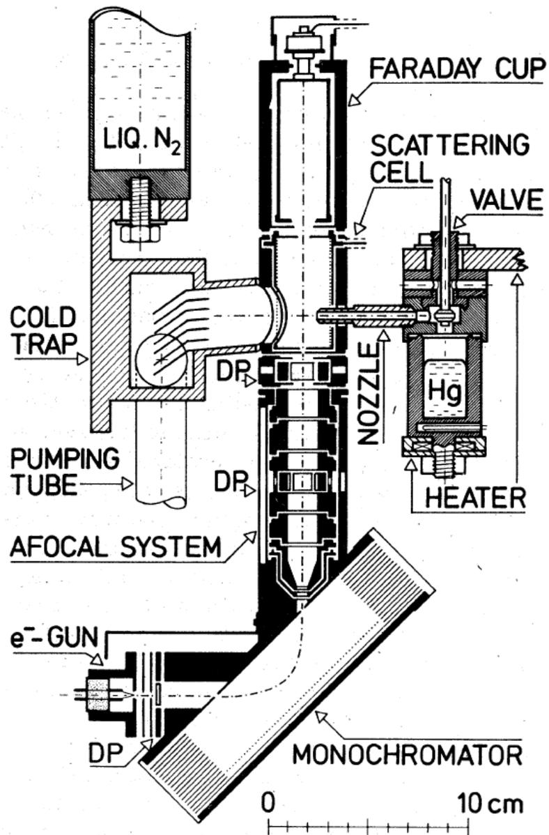
FIG. 1. Electron optical arrangement for low energy (0.1–70 eV) with atomic beam target. Deflector plates are denoted by DP.
